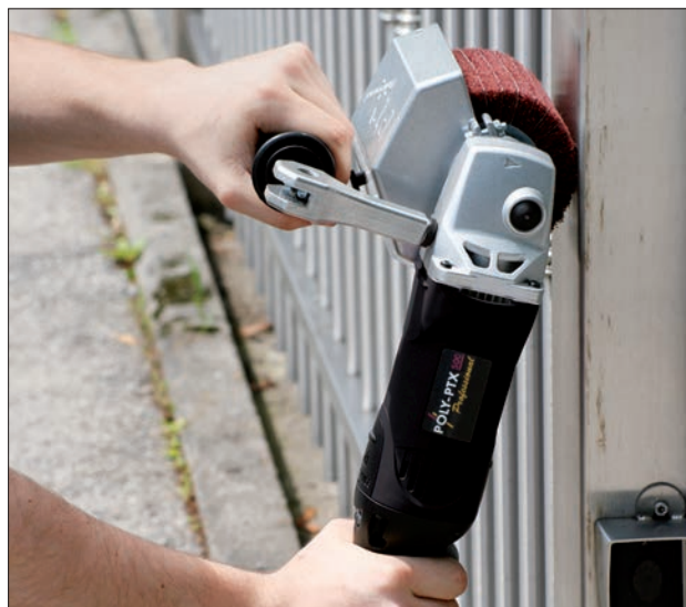
Satin finishing using interleaf fleece wheel.
